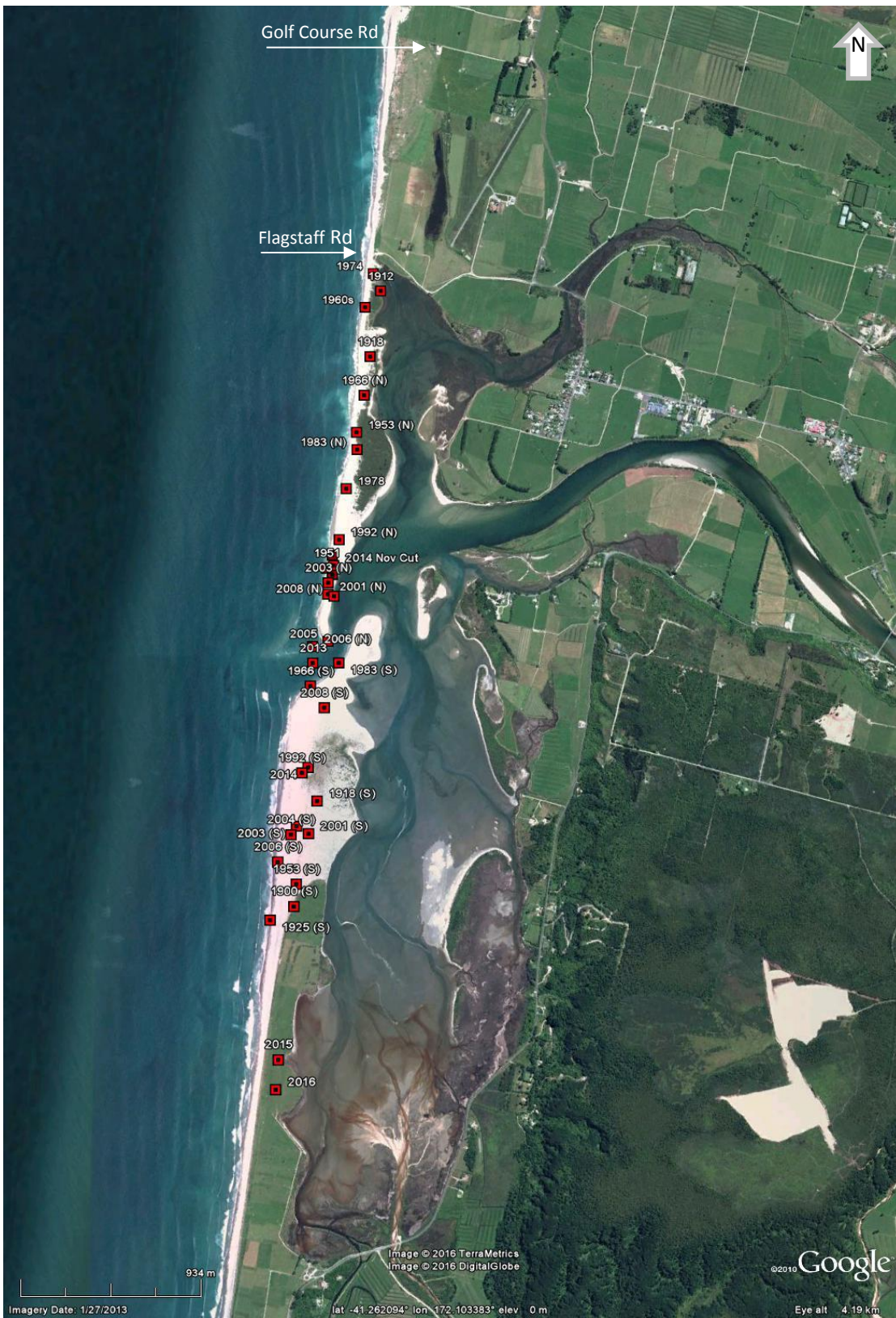
Figure 2: Location of known estuary openings. Year of observation with north (N) or south (S) shown if multiple openings visible. Symbols indicate approximate centreline of opening. [Source: Google Earth image Jan 2013].
