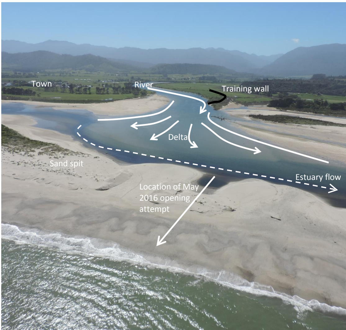
Figure 5: Aerial oblique (view to east, upriver) of Karamea River discharging into Otumahana Estuary over an estuarine delta, merging with the swamp overflow and Baker Creek (from left), before flowing south behind the sand spit (foreground). [Source: M Allis, 22-11-2016]
